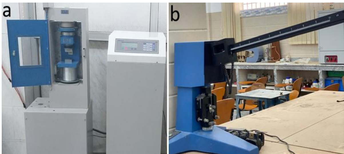
Fig. 3: a) ADR Auto compression machine with digital readout; b) Single lever flexural testing Machine
